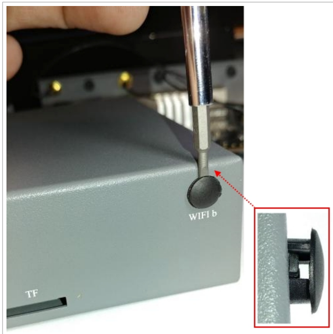
6. Removing plastic plug.png (166.26 KiB)
